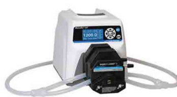
FIGURE 4: Masterflex® L/S® peristaltic pump system with two stacked Easy-Load® II pump heads connected via a double-Y tubing assembly.
